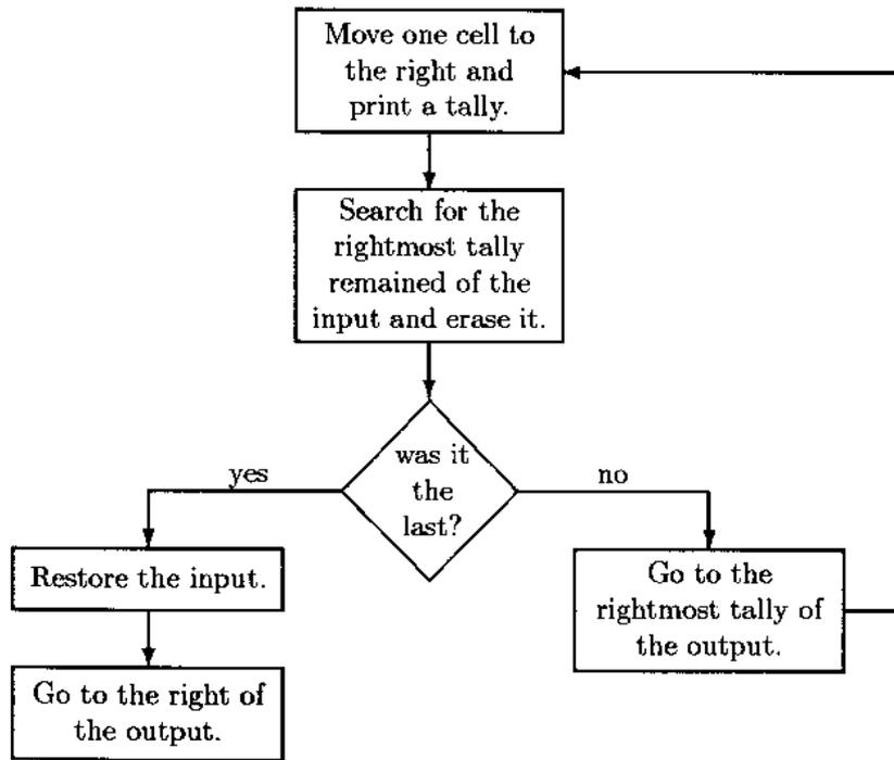
Figure I.1: Flowchart for  $T_1^1$
